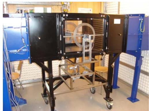
Figure 3: The closed test section with assembled measurement system in the windtunnel
