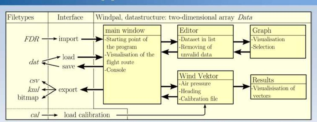
WinPal was designed as a main tool for processing the data gathered during a flight. The following windows make working with this data as easy as possible:
