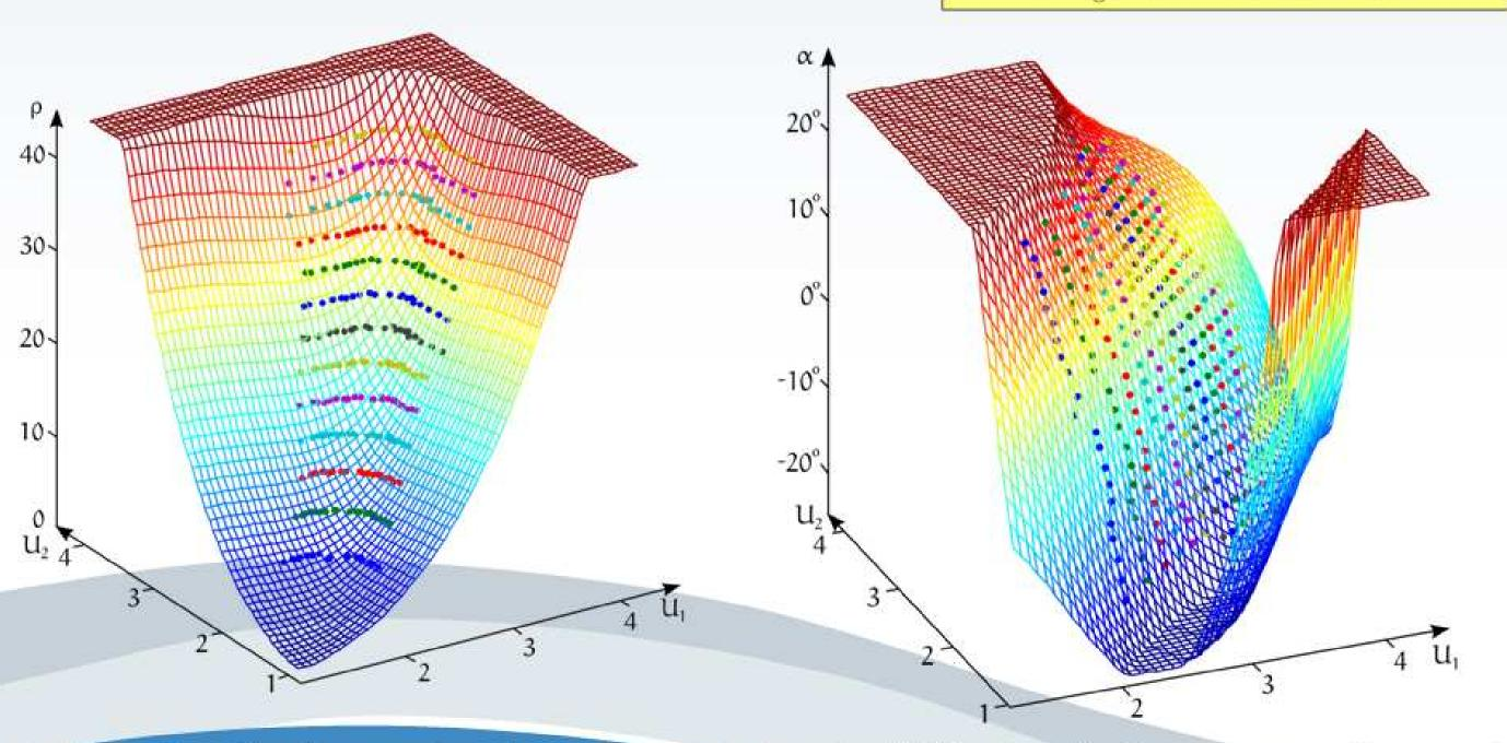
Density flow as function of sensor signals. (With density flow, temperature and Left: air pressure it is possible to calculate the Wind velocity.)
