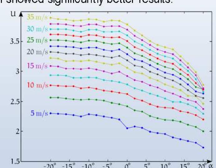
Shown above are the output signals of single sensors as a function of the angle of attack at different wind velocities. The gradient of the opened sensor (left) is considerably lower than the gradient of the closed one (right).
