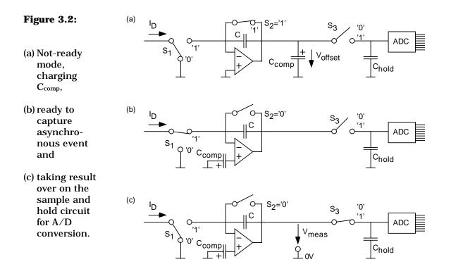
To realize the switches, advantage is taken of the fact that the MixED models allow for resistor manipulation during runtime. Simulation results are shown in Fig. 3.4.
