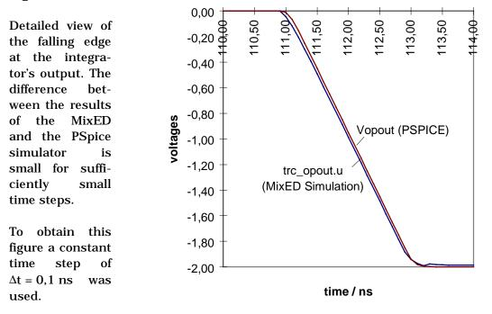
As shown in Fig. 3.5 the implicit backward Euler integration of the MixED models allows for accurate results if sufficiently small time steps are used. The numerical stability of the employed operational amplifier model according to [4] is excellent. To employ the switches in a numerically effective and stable way needs some experience. In the above simulation infinite switching speed and no need for overlapping clocks was assumed.
